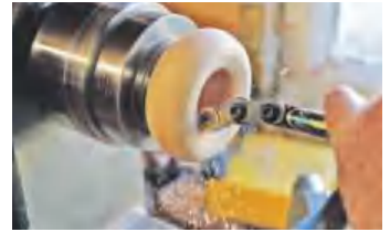
Altering the angle of attack allowed me to make controlled cuts
